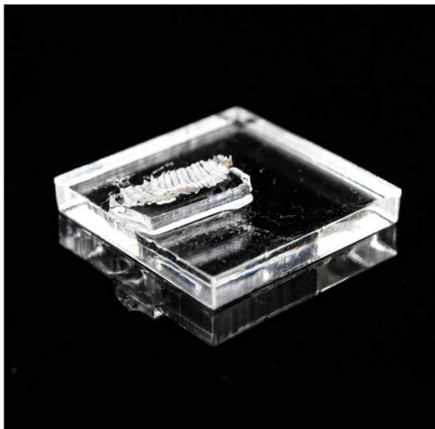
**Fig. 1** Example of a prototype physical model with the fibrillar surface pointing up and attached to a PDMS backing sized to approximate overall effective compliance of a gecko toe pad. Note that the fibrillar surface area is approximately equal to that of a single toe of a Tokay Gecko.
