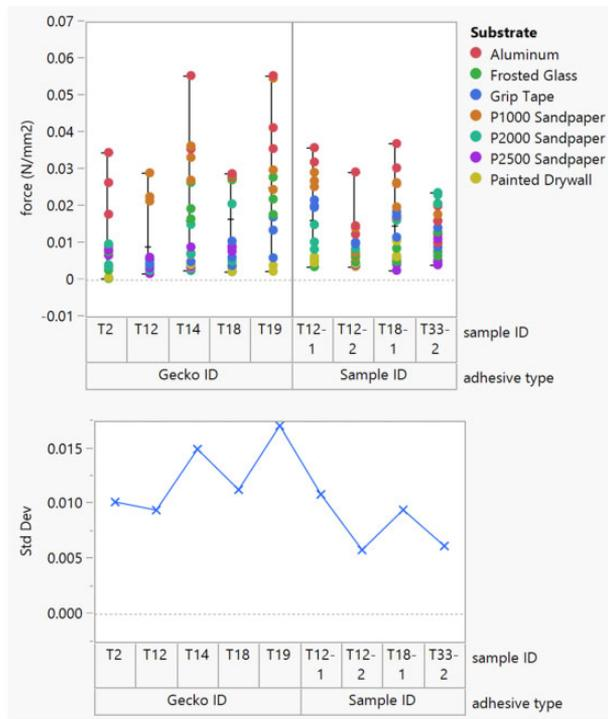
**Fig. 3** (Top panel) Variability chart of adhesive force observations of geckos and physical models, color coded by substrate type. Vertical lines show range of observations, cross-hatches show overall mean force across substrate type for each adhesive ID (individual geckos or physical models). (Bottom panel) Standard deviation of observations for each adhesive ID (individual geckos or physical models) lumped across substrate type.
