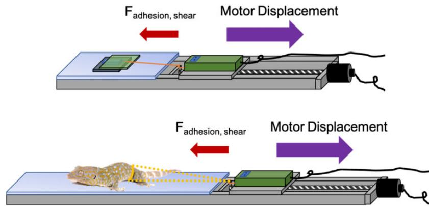
**Fig. 2** Diagram showing the horizontal force testing apparatus (Niewiarowski et al. 2008) and setup used to test adhesion of live geckos (bottom panel) and physical models (top panel).
